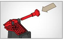
**Step 1.** Put the Pivot Pin Tool (PPT) fixture over the pin housing on the lower and insert large PPT pin.
