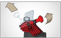
**Step 3.** Rotate the PPT assembly 90 degrees and then remove the plunger.
