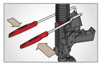
**Step 2:** Squeeze handles together to grip Delta Ring.
