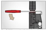
**Step 3:** While squeezing the handles, pull down to compress and disengage Delta Ring.
