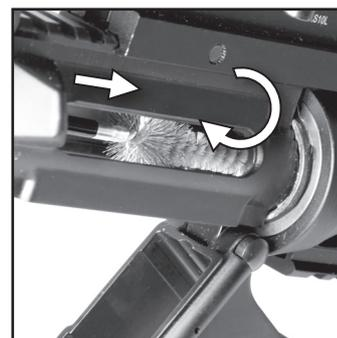
**STEP 3:** Replace the chamber brush with the male thread adaptor and a felt chamber star. Apply a few drops of solvent to chamber star. Insert chamber star and rotate clockwise to absorb the loosened fouling. Repeat this step using additional chamber stars until they come out clean.
