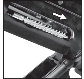
**STEP 8:** Re-attach the slotted bore patch tip to the rod (with a clean/dry patch). Push the clean patch through bore. The patch will absorb loosened fouling. Repeat steps 5 through 8 using multiple patches until the last patch comes out clean.
