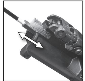
**STEP 10:** Maintaining a clean bolt carrier group is also essential to proper AR15 function. Remove any excess carbon build up using solvent along with the brushes and picks included in this kit.
