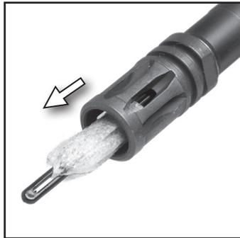
**STEP 9:** Once the chamber and bore are clean proceed to wipe down the action with a clean patch lightly coated in solvent. Stubborn fouling may be removed with nylon brush. Be sure to remove any stray fouling after brushing. Finally, wipe down action with a clean dry patch to remove any excess solvent.
