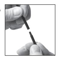
**STEP 5:** Attach the slotted bore patch tip to the end of the rod. Slide a cleaning patch through tip. Apply a generous amount of solvent to the patch.
