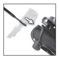
**STEP 7:** Attach the bore brush to the rod. Guide the rod and push the brush through bore from action to muzzle. This step loosens more fouling.
