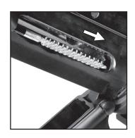
STEP 8: Re-attach the slotted bore patch tip to the rod (with a clean/dry patch). Push the clean patch through bore. The patch will absorb loosened fouling. Repeat steps 5 through 8 using multiple patches until the last patch comes out clean.
