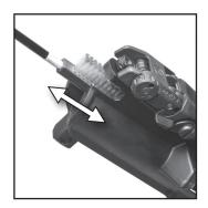
**STEP 10:** Maintaining a clean bolt carrier group is also essential to proper AR15 function. Remove any excess carbon build up using solvent along with the brushes and picks included in this kit.
