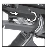
**STEP 3:** Replace the chamber brush with the male thread adaptor and a felt chamber star. Apply a few drops of solvent to chamber star. Insert chamber star and rotate clockwise to absorb the loosened fouling. Repeat this step using additional chamber stars until they come out clean.
