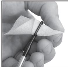
**STEP 4:** Re-attach the slotted tip or jag to the rod (along with a clean/dry patch). Push the clean patch through the bore from action to muzzle. The patch will absorb loosened fouling. Use a correctly sized mop for shotguns. Repeat steps 2 through 5 using multiple patches until last patch comes out clean.
