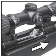
**STEP 5:** Once the bore is clean, wipe down the action and its parts with a clean patch lightly coated in gun solvent to remove any stray fouling. Finally, wipe down action with a clean dry patch to remove any excess solvent.
