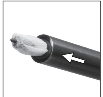
**STEP 2B - JAGS:** Pierce the center of an appropriately sized cleaning patch with the tip of the jag and wrap the patch around the jag. Apply a generous amount of gun solvent to the patch. From action, carefully guide the jag into the opening of the bore and push it the length of the bore using a consistent pressure. Extract the rod and dispose of the used patch. We do not recommend re-inserting the jag/patch multiple times. Use a fresh patch for each pass through the bore.
